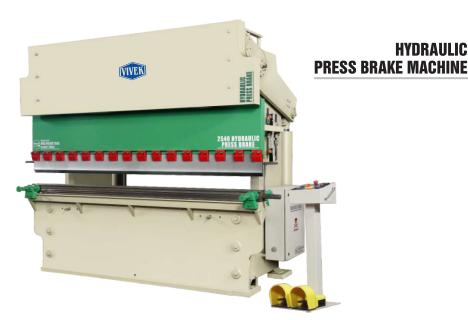
FRAME: The Frame is rigidly constructed from Solid steel plates with safeguards, It's interlocked design provides support to the bed directly on the frame to avoid weak sections at load supports.
